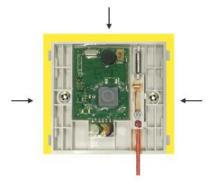
**Step 2**. Fix the bottom cover, screw the bottom cover of the button onto the embedded 86 box, tighten the screws properly, and then test the smoothness of pulling rope.
