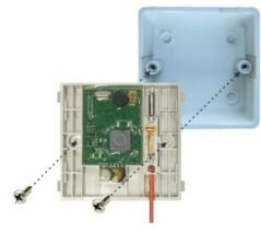
**Step 2**. Fix the bottom cover, screw the bottom cover of the button onto the embedded 86 box, tighten the screws properly, and then test the smoothness of pulling rope.
