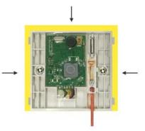
**Step 3.** Glue the upper, left and right sides of the bottom cover with water-proof glue to avoid water inside the equipment to accelerate the aging of the line; ensure that the long-term pulling of the cable causes the equipment to move, and finally fasten the cover.
